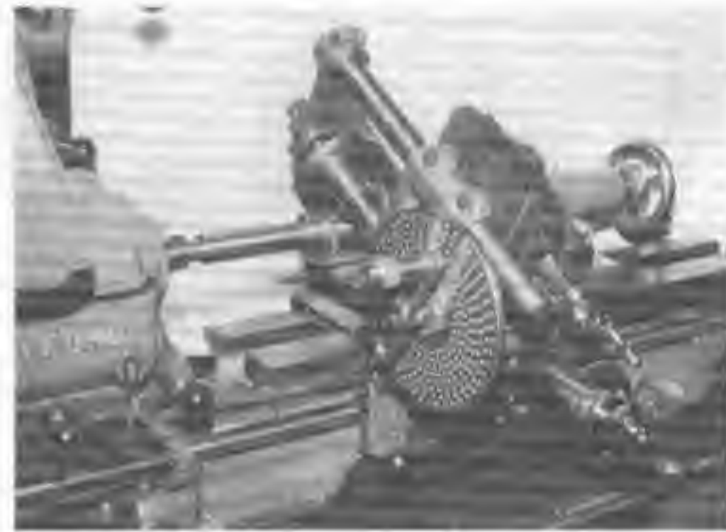
Fig. 60 This shows how the swivelling vertical slide is used to provide more headroom for the accommodation of larger gears.
